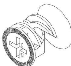
Notice the Cam Lock has a "C" Shaped Back. An arrow or +/- signs on the front indicate the open section on the back of the Cam Pin.
