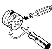
The head of the cam bolt goes into the open mouth of the cam nut. You then turn the cam nut so it tightens over the bolt.
