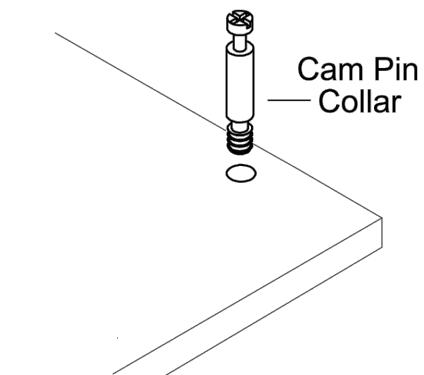
The Cam Pin is inserted into the flat side of a board, it is important that: The cam pin is kept vertical and is not put in on an angle. Cam pin is to be inserted up to collar Too far and it wont catch the Cam Lock (Do Not Overtighten) Not enough and the resulting product will not be stable.
