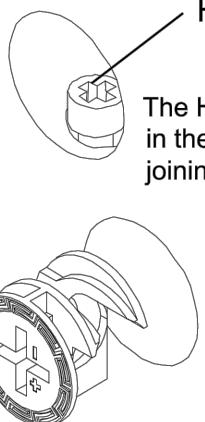
The Head of the Cam Pin will be visible in the large hole on the side of the joining board.
